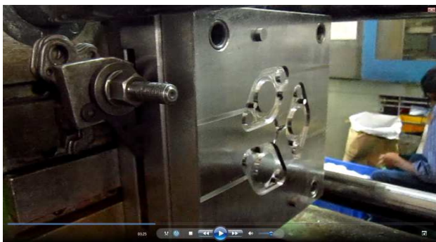
Fig.18: Tool loading into machine
